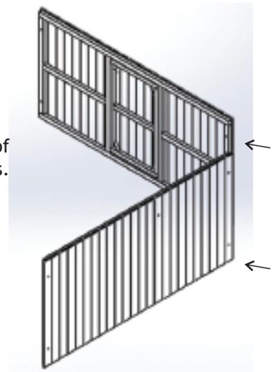
With localized parts, align the holes of the skirt with the location of the inserts.
