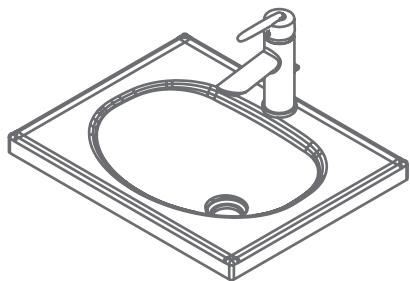
After drilling the hole, polish it with 60 grit sandpaper, proceed to install the faucet, according to the faucet's manual.
