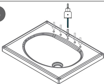
Drill the holes guided by the marks made by the drill bit, using the 1 1/4" cup saw. This should be done drilling the front side of the lavatory, repeat this process for the other holes required for your faucet. \* Lateral view of the lavatory.
