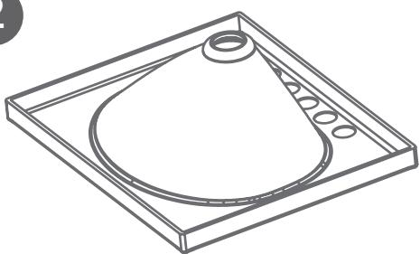
Make a small hole using the guide drill bit, aiming for the center of the hole where you want to install the faucet.
